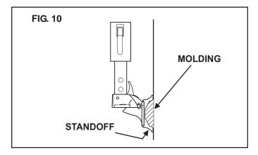
**Note:** If installing over a molding, A&E (Single) Standoff Kit 3104781.004 (Bulk 10 pack 3104781.103) may be used (See FIG. 10).
