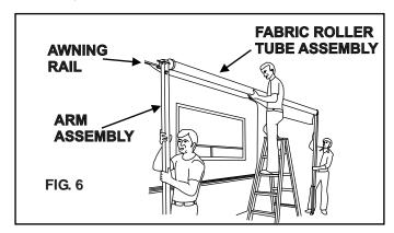
Feed the awning into the awning rail while standing on a stepladder, (third person) while two carry the awning assembly to the desired position.
