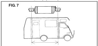
The top mounting bracket can be placed in several different positions with relationship with the awning rail. Some awning rails have a drip channel to catch water as it runs off the roof and drain it to the front or rear of the coach.
