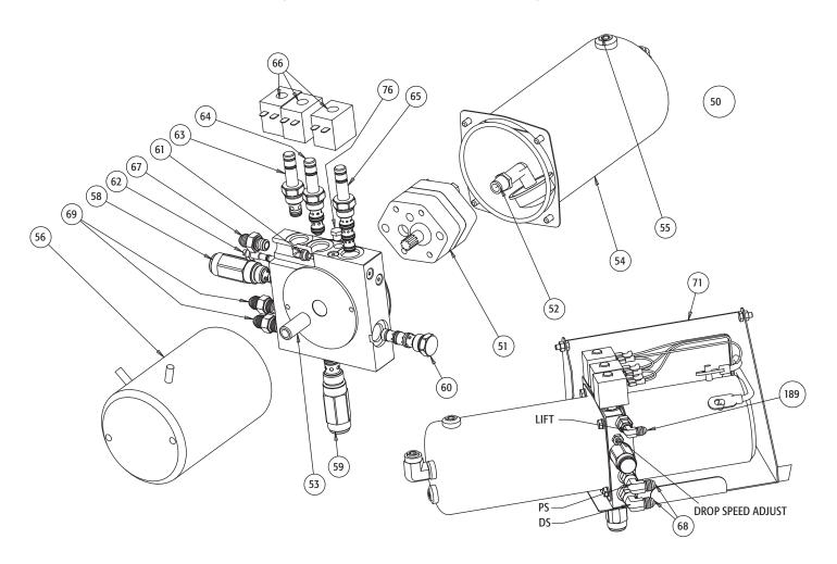
**Hydraulic Power Unit Wiring**
