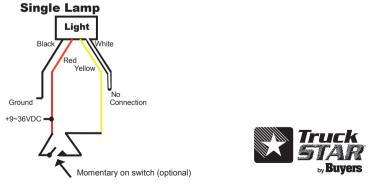
Make connections as in Step 1 & 2. The white wire is not used for a single lamp installation.
