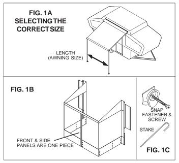
The above-mentioned panel and skirt are secured to the vehicle, the awning and to the ground by means of zippers, snap fasteners, PE clips, and hook stakes (provided). See FIG. 1C.
