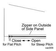
**NOTE:** For adjustable pitch awnings, it may be necessary to adjust the pitch of the awning so that the panels hang straight.
