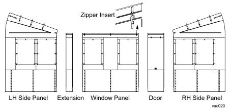
The front panel sections include a removable top piece called the zipper insert. For convenience, the zipper insert can be removed and slid into the lead rail or roller tube. Then the panel can be lifted and zipped to the insert.
