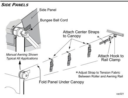
If not previously done, insert the bungee ball through the grommet located in the front upper corner of the side panel. The cord should be inserted from the outside face of the panel.
