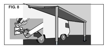
Important: Never leave the roller tube level with the awning rail, adjust both arms of the Universal Hardware 7 to 8 adjustable arm holes below awning rail (fabric slope approximately 10 degrees). Sunchaser hardware should be in the water shed position. See FIG. 9.
