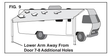
**Note:** Universal hardware is designed with a water dump feature that will lower one side of the awning to allow water to run off. Before the water dump feature will operate as designed, lower both arms 7 to 8 holes (fabric slope approximately 10 degrees) below the coach awning rail. The water dump feature will not work if awning is flat. See FIG.
