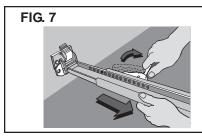
Pull Up On Handle To Release Lock Button, Lower Handle to Engage Button
