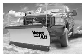
plow path, in the angled position, should exceed the tire track by at least six inches on either side. Be sure to have enough slack in the lift chain while plowing so the cutting edge of the moldboard can follow the ground contour. Use the adjustable runner shoes to set the bottom edge of the plow just above the ground for best operation.
