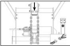
Lower Plow to float position and manually push lift arm down. Disconnect the electrical connection.
