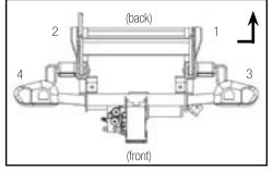
Pull, then rotate blue pins on both sides of truck into locked out position. The vehicle is now free from mount and may safely back away.
