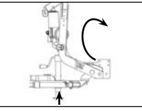
2 Rotate blue pins until engaged and push top of lift frame towards truck until pins click in place.
