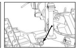
2 Remove crankstand from storage position on the side of mount and reattach to "A" frame. Crank until front of truck rises slightly.
