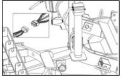
Return crankstand to storage position and reattach the electrical connection. The mount is now securely attached to the vehicle and is operational.
