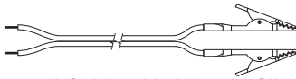
Universal Cable with Alligator Clips for External Emergency Terminals or Motor Cables with Quick Disconnects
